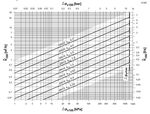
$\Delta p_{\text{max}}$  = Maximum permissible differential pressure over the valve control path, valid for the entire positioning range of the valve-actuator unit:
